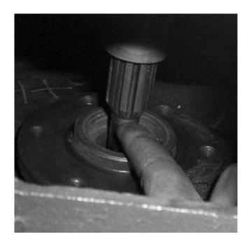
NOTE; IN CERTAIN SITUATIONS IT MAY BE NESSECARY TO SHORTEN THE TRANSMISSION FRONT BEARING RETAINER. THIS CAN BE CHECK BE INSTALLING THE FLYWHEEL AND CLUTCH DISK ONLY, THEN WITH THE TRANSMISSION INSTALLED THE CLEARENCE BETWEEN THE CLUTCH DISK HUB AND THE TRANSMISSION BEARING RETAINER CAN BE CHECKED. IT SHOLD BE A MINIMUM OF 1/8".
