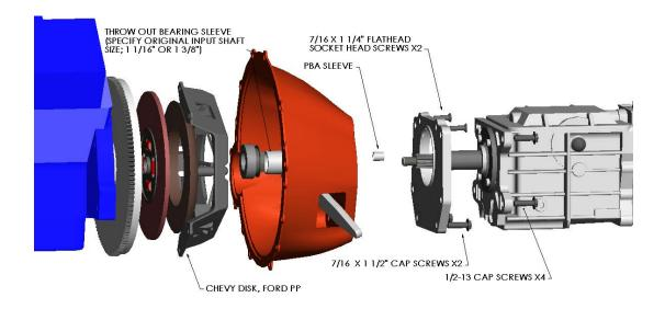
PLACE THE ADAPTER PLATE ONTO THE BELLHOUSING. IF NECESSARY USE A RUBBER MALLET TO FIT THE PLATE UP FLUSH. INSTALL THE SCREWS USING A THREAD LOCKING COMPOUND AND TORQUE. NOTE; IF YOU ARE USING THE 49-53 FORD STAMPED STEEL BEELHOUSING, THE FLATHEAD SOCKET HEAD CAP SCREWS MUST BE SWITCHED TO 7/16-20 SCREWS. DO NOT USE THE CAP SCREWS TO FORCE THE PLATE ONTO THE BELLHOUSING. MAKE CERTAIN THE ADAPTER PLATE SITS FLUSH TO THE BACK OF THE BELLHOUSING AND THERE IS NO GAP.
